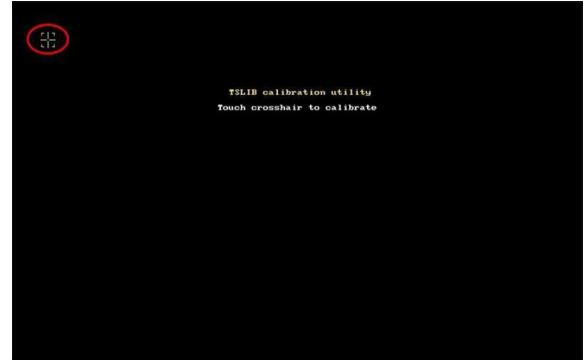
※ During the correction, please do perform the operation according to the positions of crosses. Otherwise, the touching panel will be unable to work normally after the correction.
