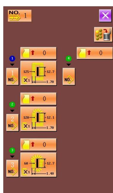
The right figure is the edition on the data of the continuous stitching. On specific operation, please refer to Continuous Sewing Data Input.
