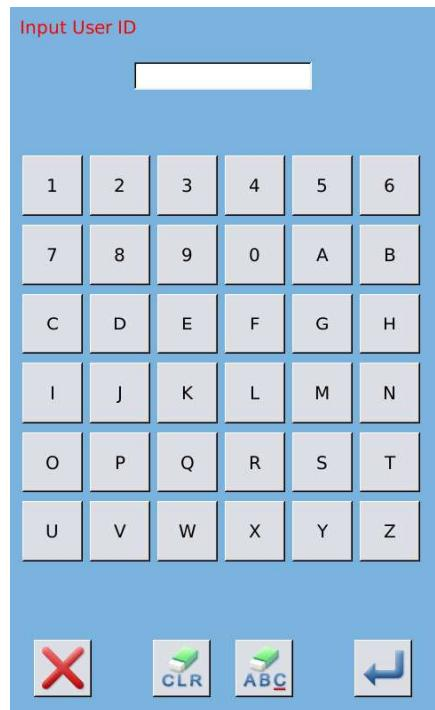
③ Input the Correct Factory ID to enter the password setting interface
